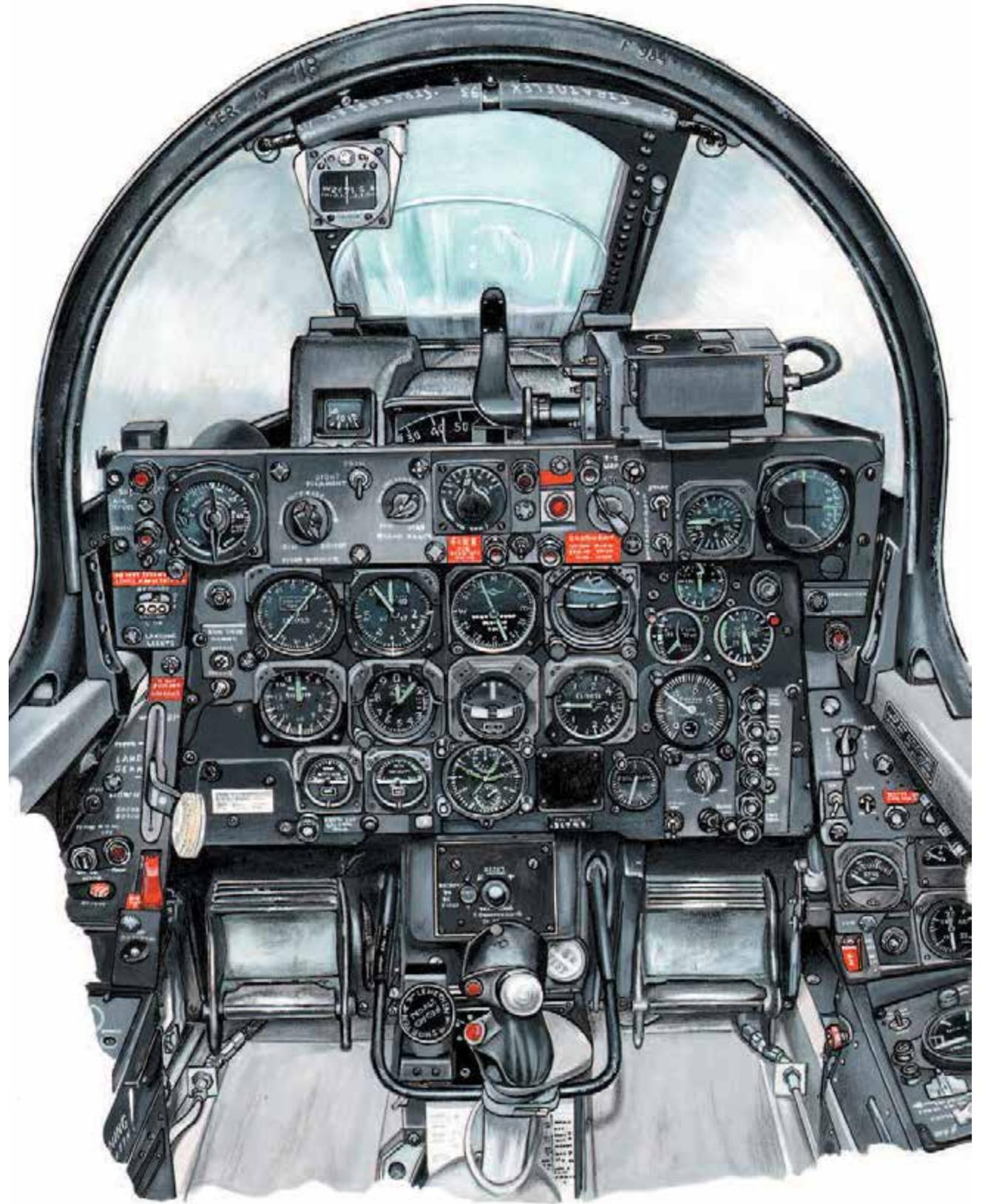
*The F-84F cockpit which was subsequently modified with different batches coming off the lines.*
